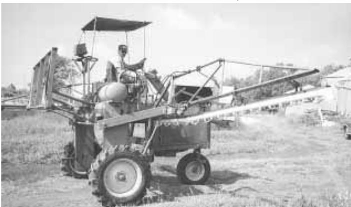
The frame that supports the 30-ft., five-section wick is built from 2 by 6-in. steel tubing.
