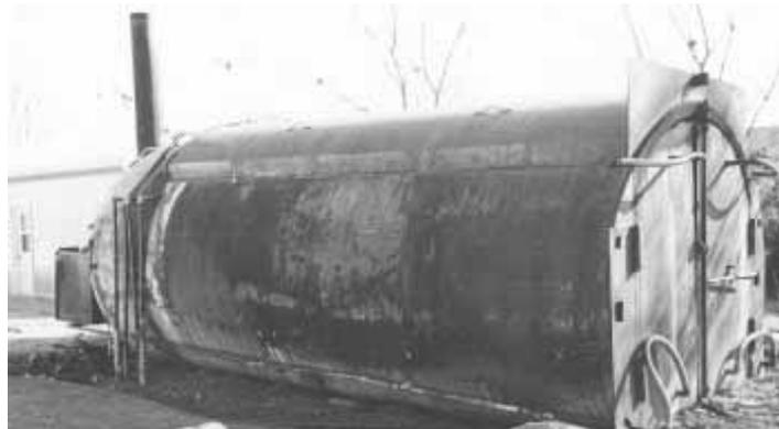
Grimm built his burner from a 26-ft. long, 10-ft. dia. section of a 60-ft. tank car.
