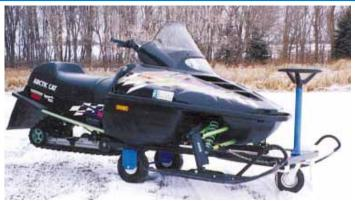
The "SnowVer" is a "pallet fork" that fits under the front end between the skis. It's fitted with two 10-in. dia. wheels that "walk" from front to back of forks to lift sled. Easy New Way To Move Snowmobiles
