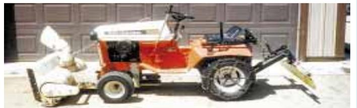
Larkin mounted blade on rear of his Allis-Chalmers 416 garden tractor which is fitted with a snowblower on front. "I use the snowblower to clear snow in one direction, then come back with the blade in the opposite direction," he says.
