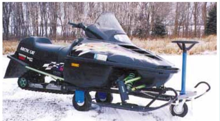
The "SnowVer" is a "pallet fork" that fits under the front end between the skis. It's fitted with two 10-in. dia. wheels that "walk" from front to back of forks to lift sled.
