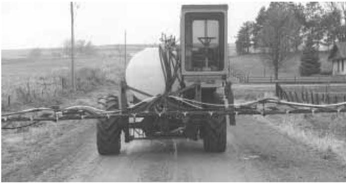
Brown used a 1959 701 Uni-Harvester to build his self-propelled "Spraymaster".
