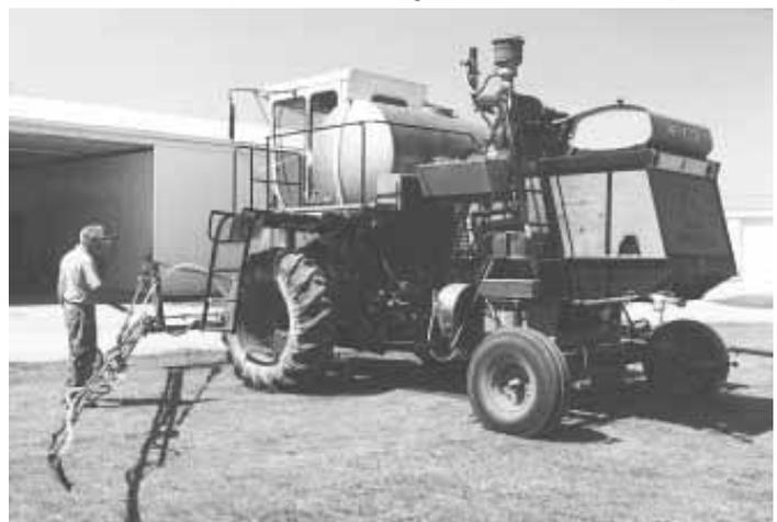
The 54-ft. boom has nozzles on 20-in. spacings for broadcasting pre-emerge and post herbicides on beans and corn. Wings are 21 ft. wide; middle section 12 ft. wide.
