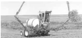
The 45-ft.boom is folded for transport by four hydraulic cylinders.
