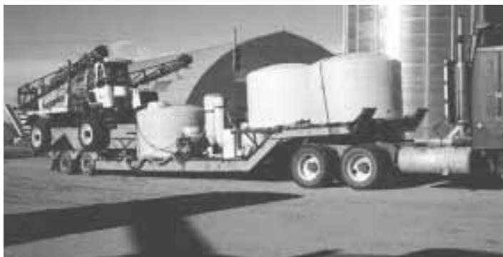
In addition to the Weisz' sprayer, the trailer hauls three 1,550-gal. tanks, three 100-gal. mini tanks, a measuring tank, and various chemical and rinse tanks.
