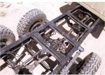
He mounted an extra transfer case 2 1/2 ft. behind the cab, positioned so it faces backward. A pair of driveshafts on the transfer case are used to power the mid and rear axles, with one driveshaft going to each axle.
