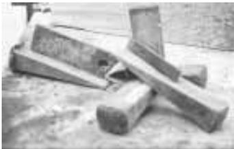
**Roland Holder, Hinton, Iowa:** "I keep a few old wood splitting wedges on my welding bench to hold uneven pieces as I weld them together. They're heavy enough to hold the parts in place and you can set up many angles. They'll adapt to most any project."
