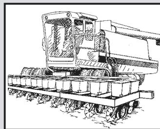
Row units attach to the combine in place of the head. Seed is stored in the grain tank and is delivered by air conveying system.
