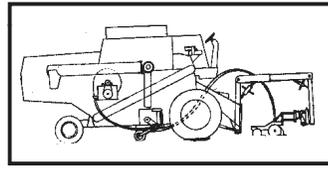
The grain tank on this combine served as a giant seed hopper, with a Wil-Rich air system carrying seed to row units up front (Vol. 6, No. 3). It was put together in 1982 by three agricultural engineering students at Iowa State University in Ames.
