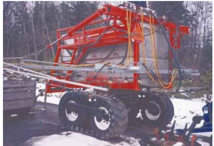
The 75-ft. wide sprayer rides on 15-in. wide, 50-in. long Goodyear rubber tracks that wrap around two 20.8 by 38 tires on each side.
