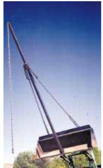
The 15-ft. long boom mounts on loader bucket to extend its lifting ability, in effect creating a miniature crane.
