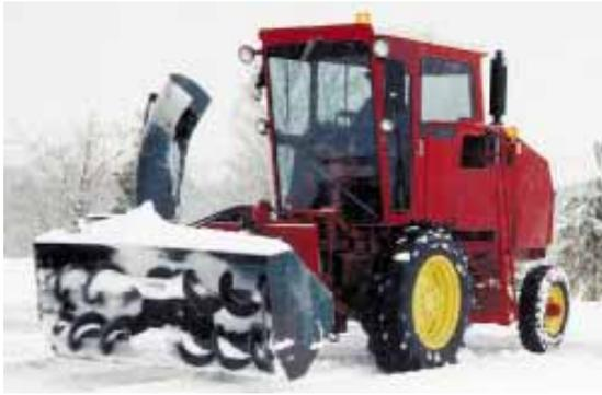
Self-propelled rig is shown here equipped with a 7-ft. wide double auger blower that's driven by a 4-speed truck transmission.
