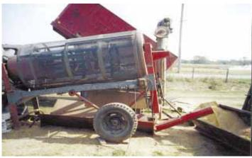
Two-stage auger system automatically dumps screenings into a big tractor bucket.
