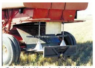
System utilizes the combine's existing spreaders and mechanical drives. Chaff And Straw Spreader For Case-IH Combines
