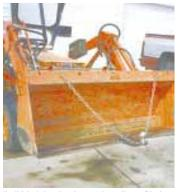
Ball hitch lets bucket push trailers. Chains can be used to support hitch.
