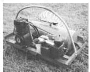
A 50 cc gas engine is used tobelt drive a single cylinder air compressor pump that pressurizes a small air tank. An angle iron frame supports all components.
