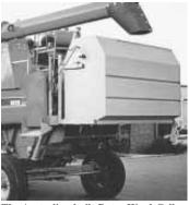
The Australian-built Rytec Weed Collection System collects weeds in a hopper on back of combine.
