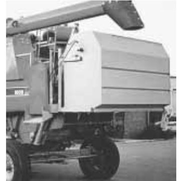
**The Australian-built Rytec Weed Collection System collects weeds in a hopper on back of combine.**
