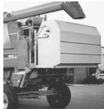
**The Australian-built Rytec Weed Collection System collects weeds in a hopper on back of combine.**
