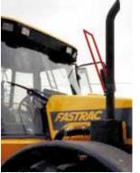
"Eyesite" mounted parallel to windshield on Fastrac tractor.
