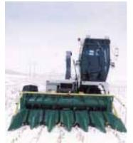
Head was built out of two used 4-row, 30-in. Deere "stalker" heads.
