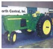
Deere 3010 repowered with Cummins 4-cyl. 4B3.9 diesel.
