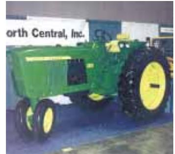
Deere 3010 repowered with Cummins 4-cyl. 4B3.9 diesel.
