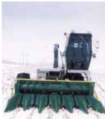
Head was built out of two used 4-row, 30-in. Deere "stalker" heads.
