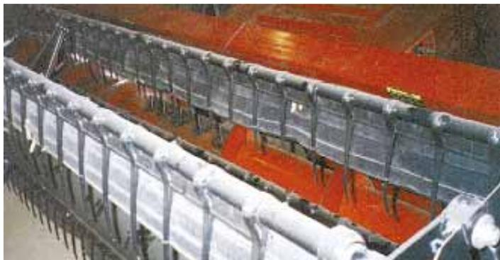
I converted the finger pickup reel on my Case-IH 1020 floating header into a modified bat pickup reel for cleaner combining in short soybeans.
