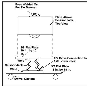
pieces of 3/8-in. thick steel plate - one 18 by 18 in. and the other 10 by 10 in. I welded a scissor jack between the two plates. Four swivel casters under the bottom plate let me roll it all over the shop. A 1/2-in. drive ratchet raises and lowers the jack easily even with a transmission resting on it. I welded eyes to the sides of the top plate for tie downs.
